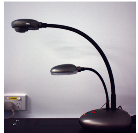
A Lumens Document Camera used to project texts and objects onto the 2Touch interactive whiteboards and Samsung plasma
